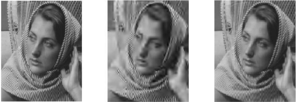
(a) Original Image (b) Compressed with 0.1bpp (c) Downsampled Image (0.8)
