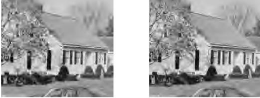
Figure 4-9 House image compressed with 0.1 bpp (left) and super resolution output (right)
