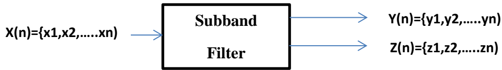
Figure 2-3 Block diagram of Subband filtering
