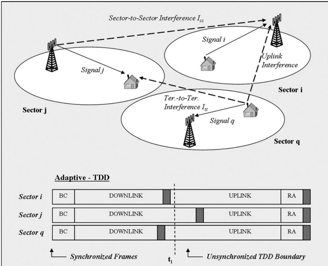
Fig: Directions of Interference in ATDD Systems<sup>25</sup>
