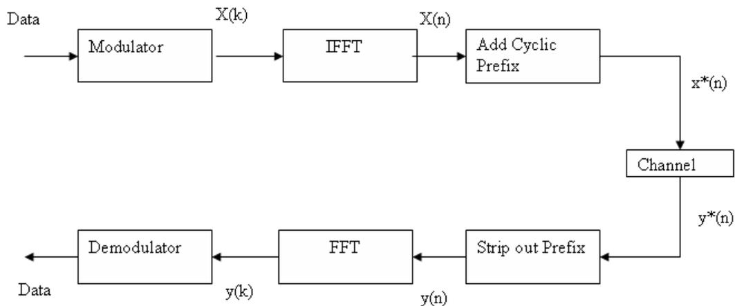
Fig: Block Diagram of an OFDM Transmitter and Receiver using Fast Fourier Transform
