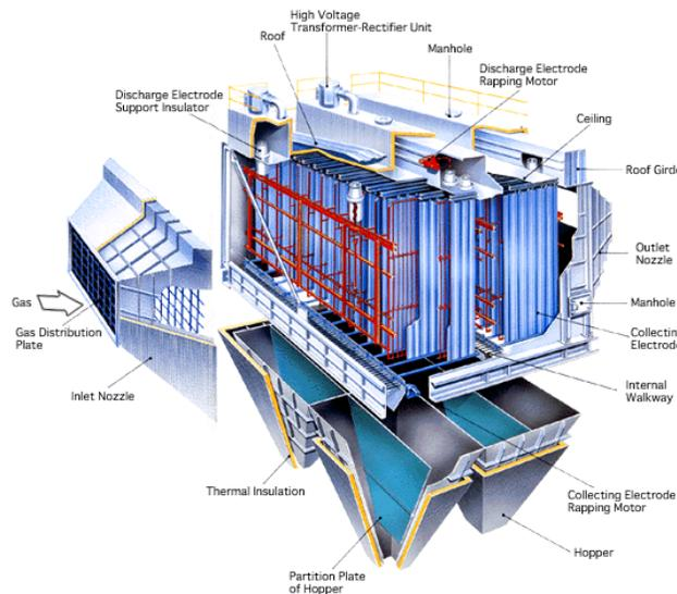
**Figure 1.7: Typical Electrostatic Precipitator Box**
