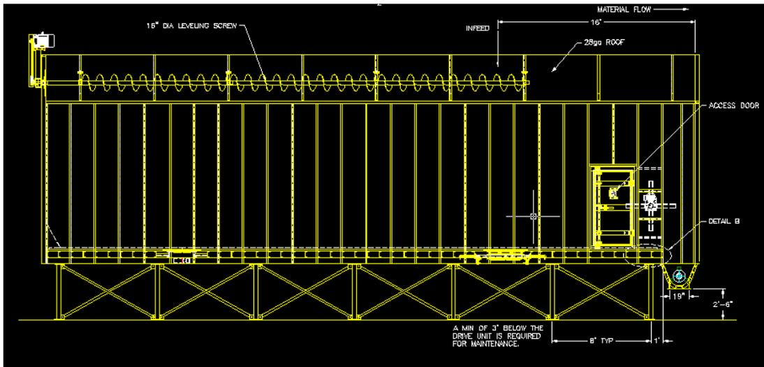
**Figure 1.4: Storage Bin with Walking Floor and Metered Screw Feed Configuration**
