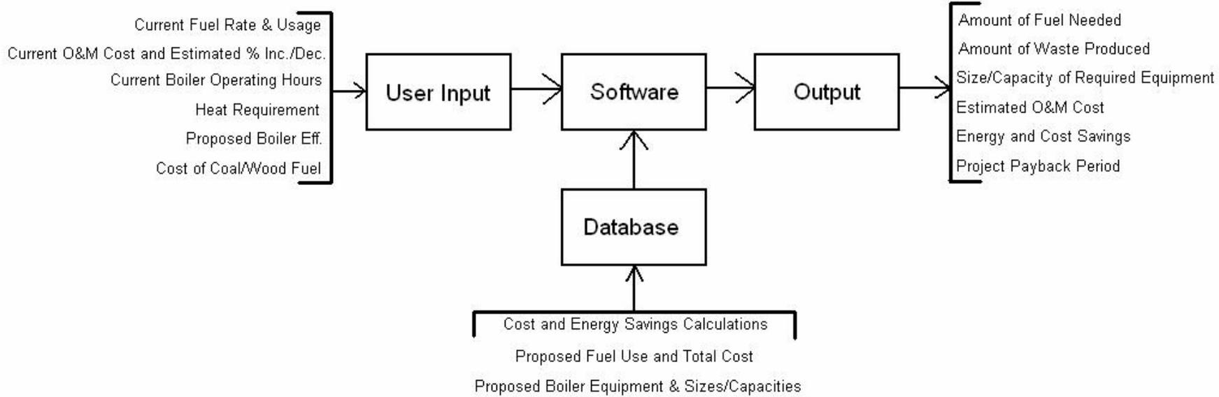
**Figure 1.9: Process Diagram for Computer Software Program**
