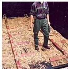
**Figure 1.6: An Example of a Walking Floor Feed System**
