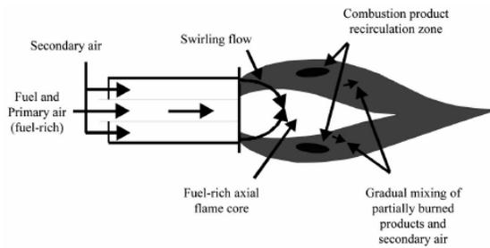
**Figure 1.8: Schematic Diagram of a low-NO<sub>x</sub> Burner**
