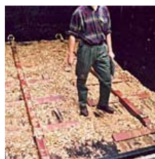
Figure 1.6: An Example of a Walking Floor Feed System
