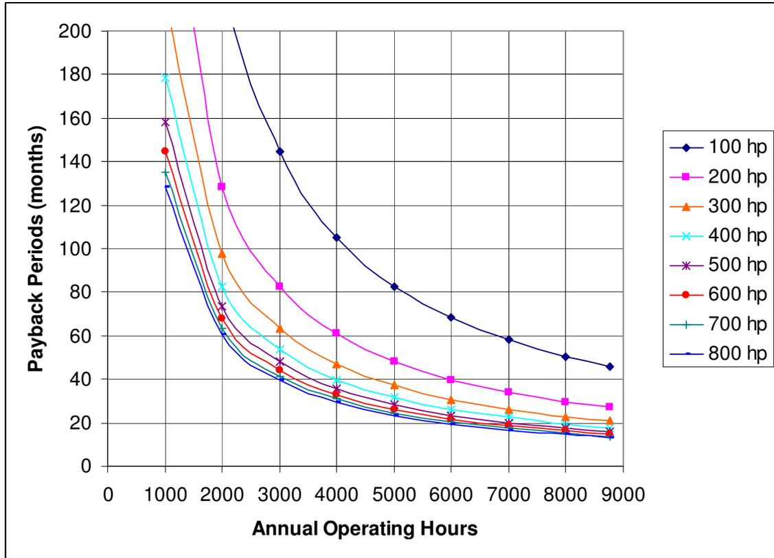
**Figure 4.7: Plot of Boiler Size and Annual Operating Hours vs. Project Payback Period**
