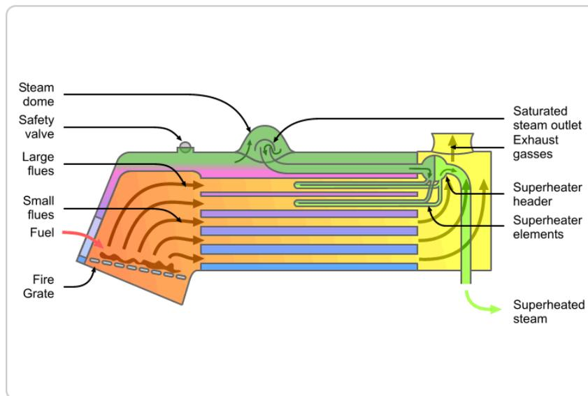
**Figure 1.2: Schematic Diagram of a Horizontal Fire-Tube Boiler**
