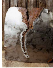
Figure 2.2: Example of Steel Corrosion
