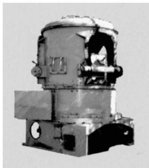
**Figure 1.3: Picture of a Typical Coal Pulverizer**
