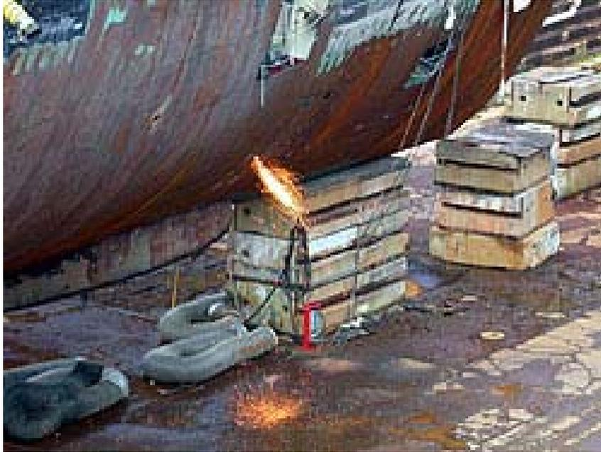
**Figure 4: Ships hull being cut using an oxy-acetylene flame (Source: [http://www.osha.gov/SLTC/etools/shipyard/ship\\_breaking/hotwork/index\\_hw.html](http://www.osha.gov/SLTC/etools/shipyard/ship_breaking/hotwork/index_hw.html))**
