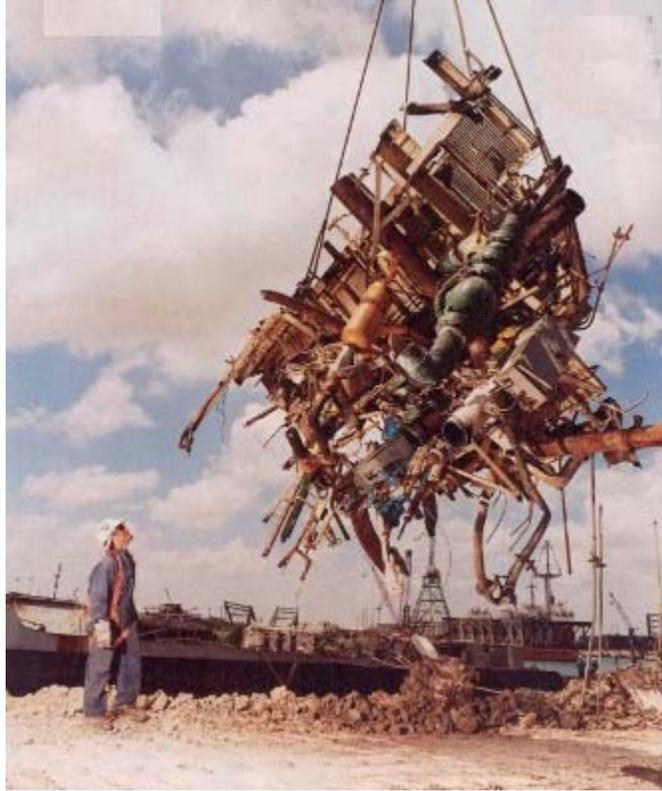
**Figure 5: Blocks of ship being removed (Source: <http://www.usshorne.net/horne/breaking.htm>)**
