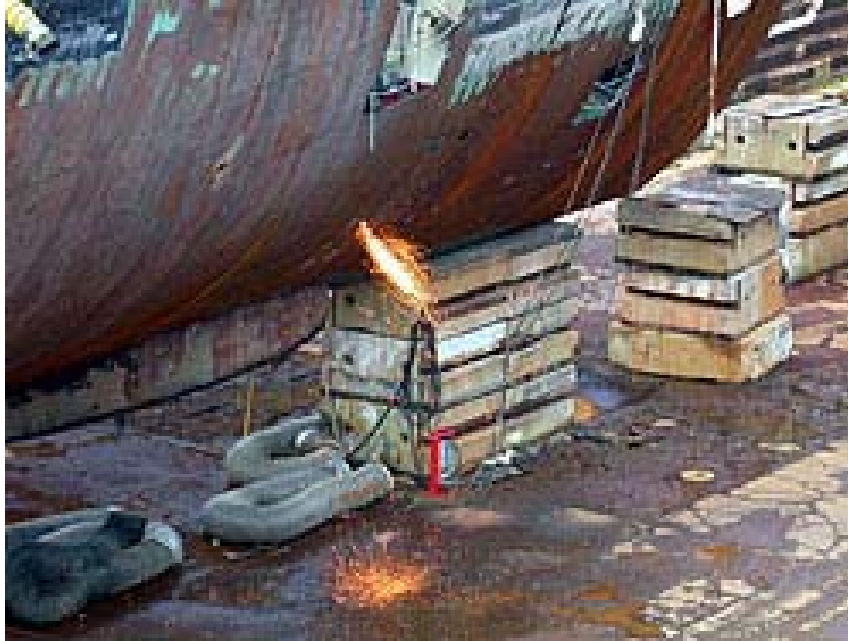
Figure 4: Ships hull being cut using an oxy-acetylene flame (Source: http://www.osha.gov/SLTC/etools/shipyard/ship_breaking/hotwork/index_hw.html )
