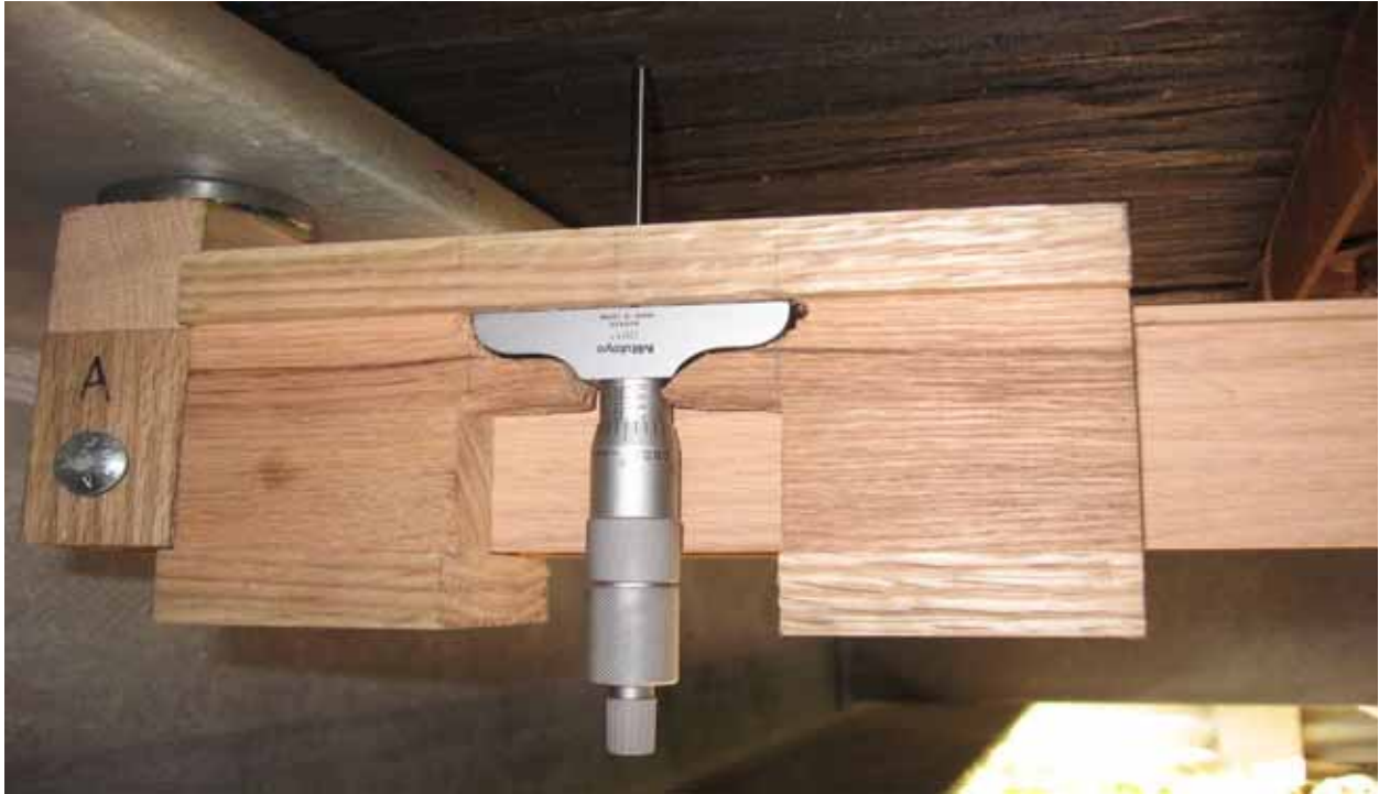
Figure 3.14: Using the Micrometer to Take Creep Measurements
