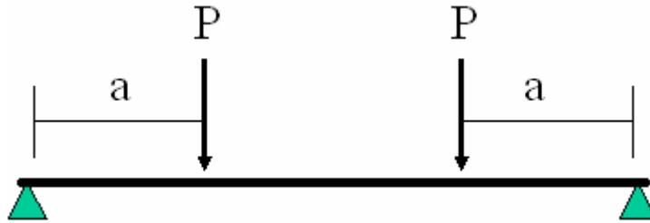
Figure 2.3: Four point bending setup (smith, 2003).
