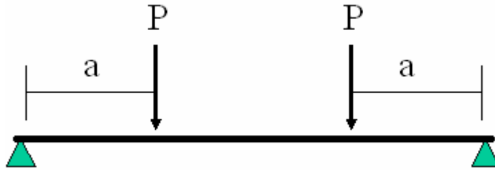
Figure 2.3: Four point bending setup (smith, 2003).
