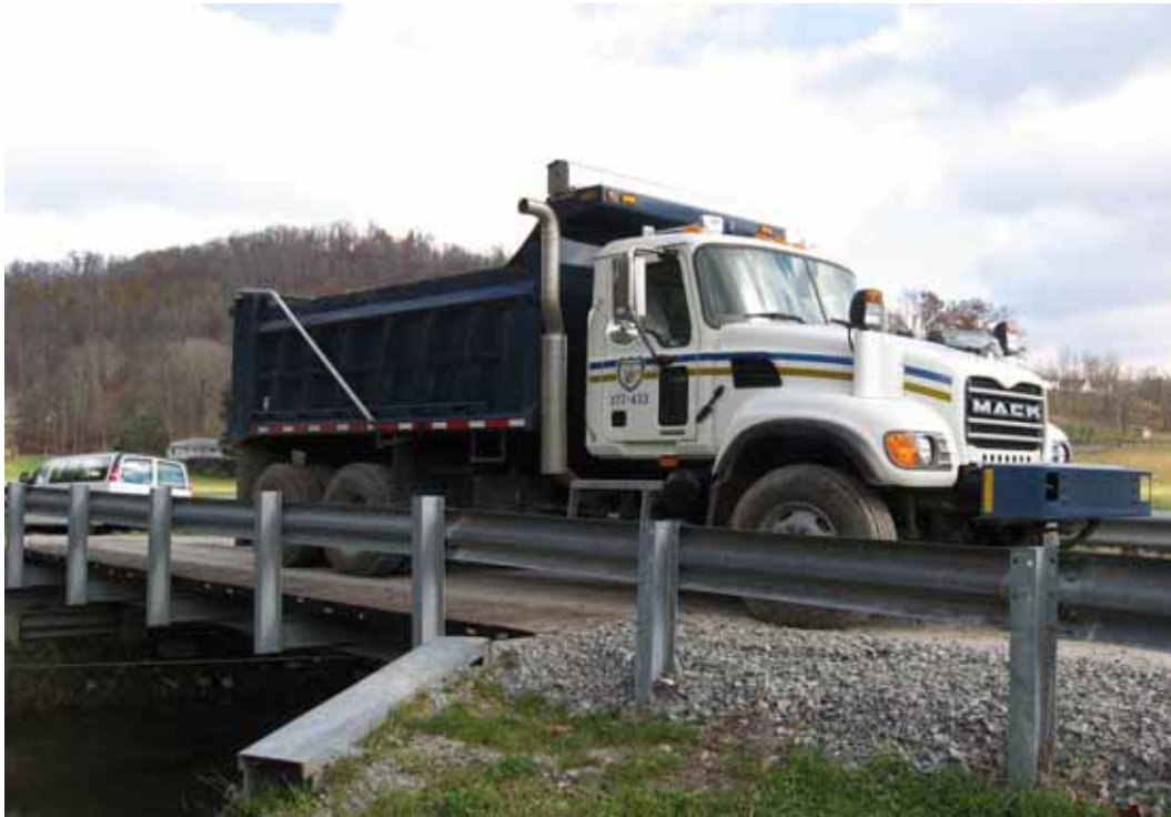
Figure 3.3: Static Live Load Test of Peel Tree Bridge
