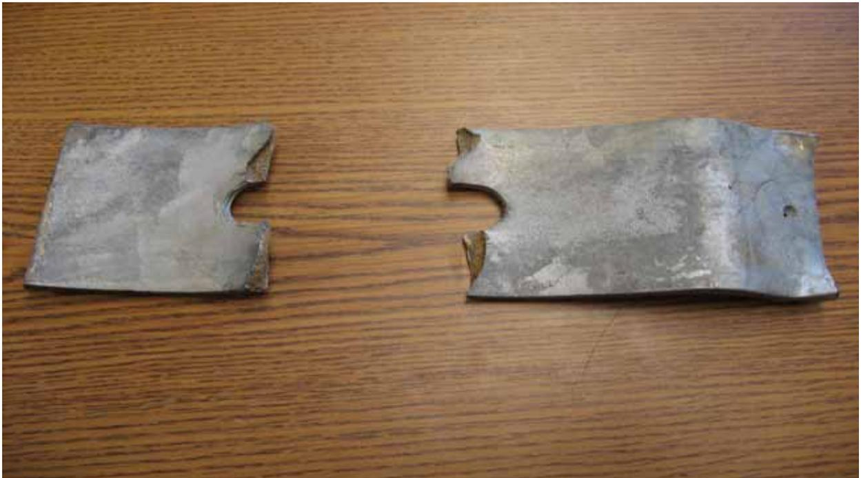
Figure 3.17: Failure Mode of a Stringer to Deck Connector on Hackers Creek Bridge
