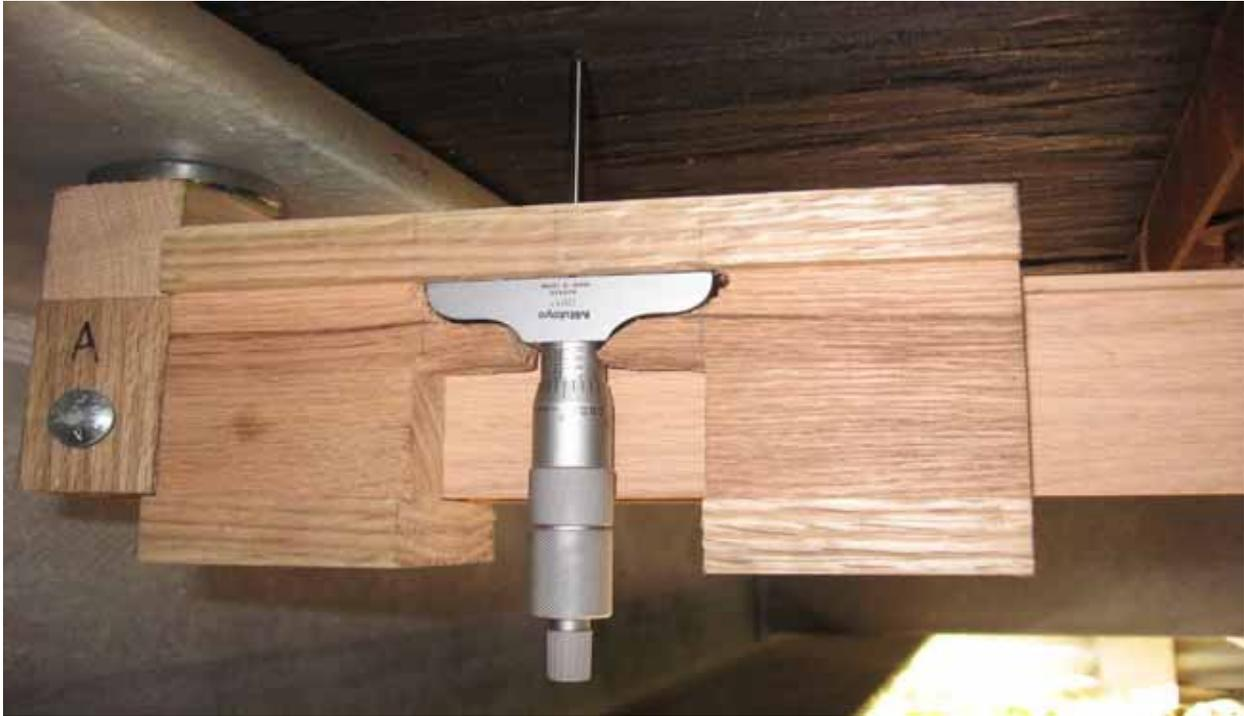
Figure 3.14: Using the Micrometer to Take Creep Measurements
